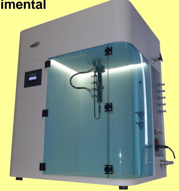
The experiments were carried out with the commercial available device dynaSorb BT Quantachrome Instruments at 40 °C. This device is designed for dynamic test routines under process relevant conditions.
