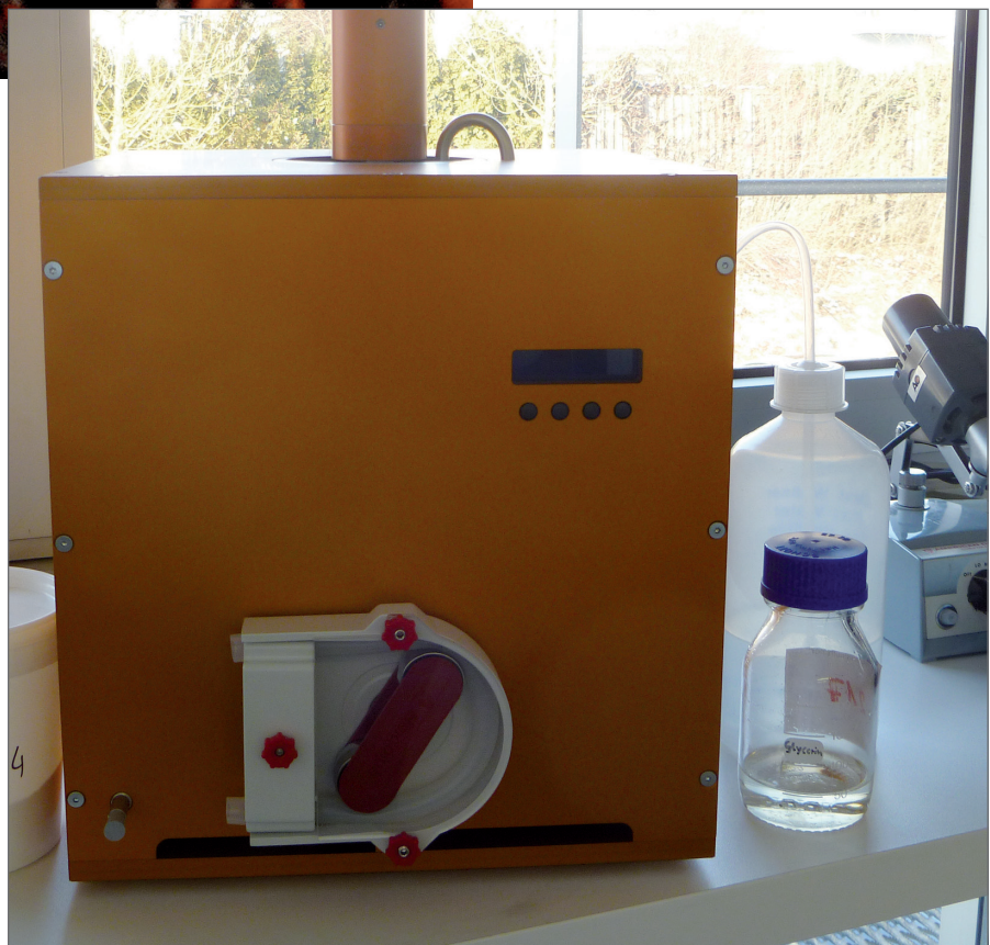
Figure 3 DISPERSER QC2 – the external dispersion unit with integrated stirrer, ultrasonic bath and circulation pump system is combinable in principle with any analyzer for the characterization of suspensions, front view (below) with peristaltic pump, display and operating buttons and plan view (above) with ultrasonic bath and stirrer
