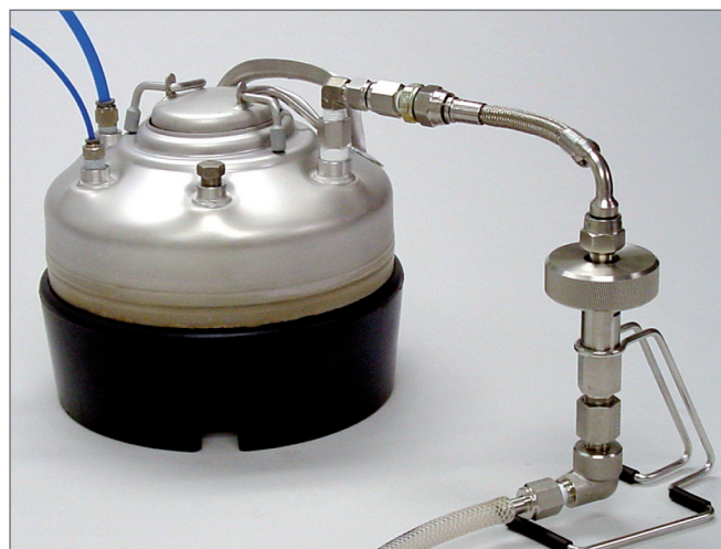
Figure 3 Option for the determination of the liquid permeability by use of the POROMETER 3G instrument series
