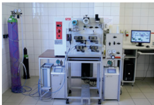
Figure 3 Self-developed RS-PPD-01 universal permeameter from GEOCHEM Ltd.
