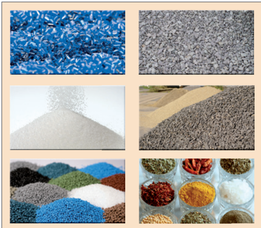
Figure 2 Powders, granules and bulk solids as possible sample types for the particle characterization with the ZEPHYR ESR (from left to right, top down): shredded plastics, fine crushed rock, sugar, various pellets, plastic granules, spicery, resp. sliced plant parts)
