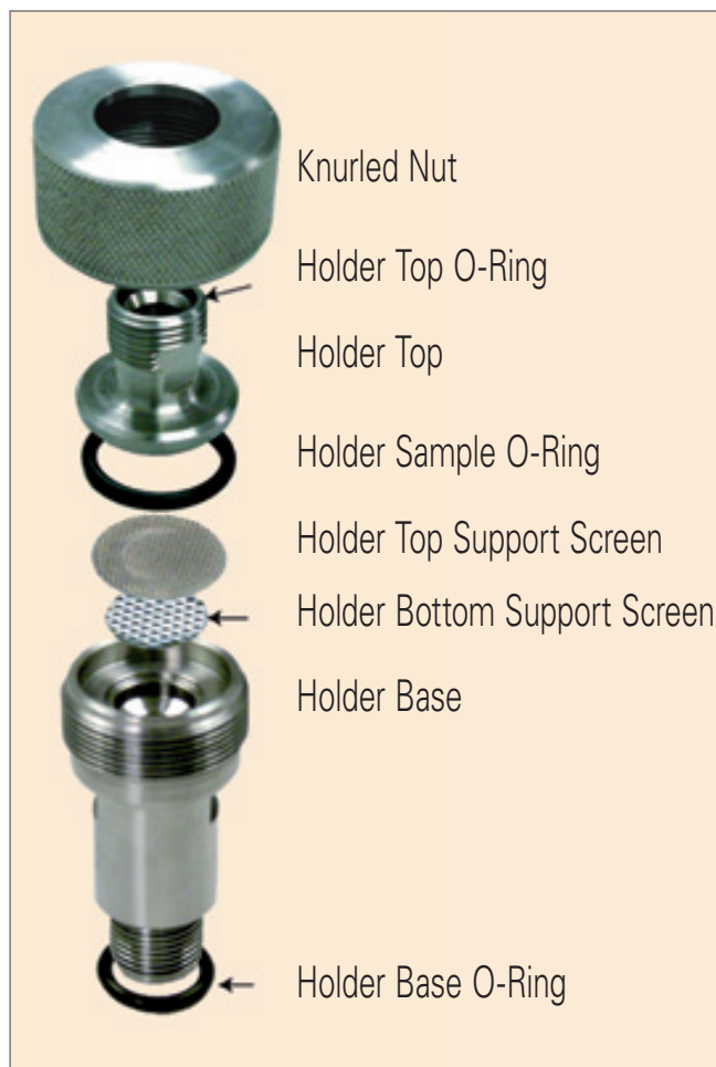
Figure 5 Open sample holder of the POROMETER 3G for flat filter samples
