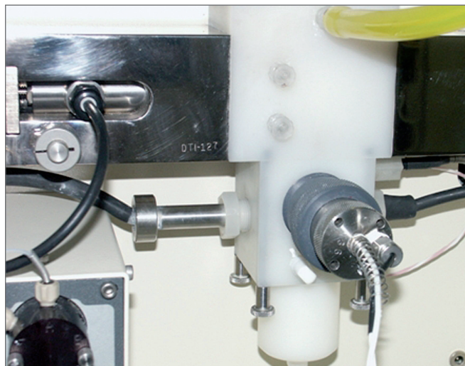
Figure 2A and 2B DT-1200 with acoustic (particle size) and electroacoustic (zeta potential) method: the zeta potential probe can be used for external experiments, like special titrations or online-monitoring (left); DT-1200 (right) with acoustic (upper block), electroacoustic (zeta probe in centre) and sensors for temperature, conductivity measurement and titration.
