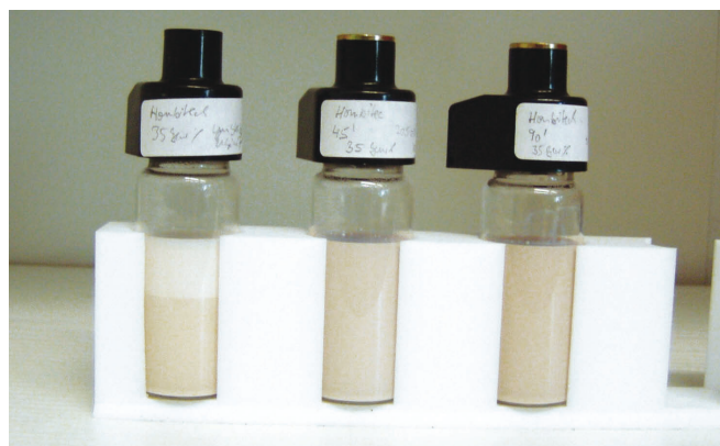
Figure 4.4 Photos of the three samples from the figure 4.3 after 30 hours sedimentation
