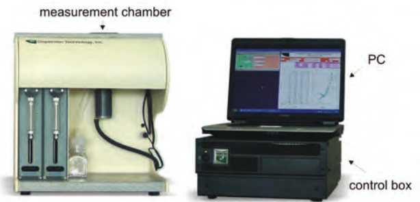
Figure 1 Acoustic rheometer DT-600
