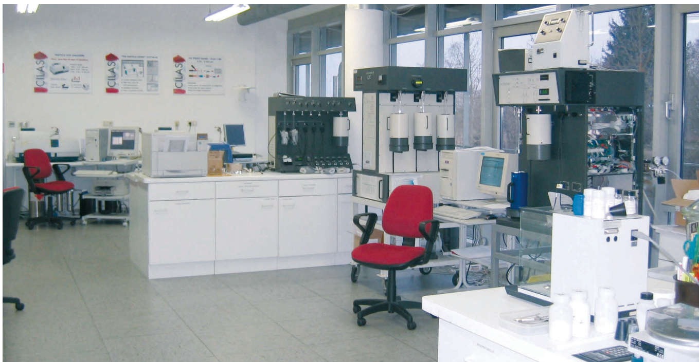
Figure 2 Partition of our Laboratory for Scientific Particle Analysis with the AUTOSORB series (right) for surface and pore analysis by gas adsorption and CILAS laser diffraction particle sizers
