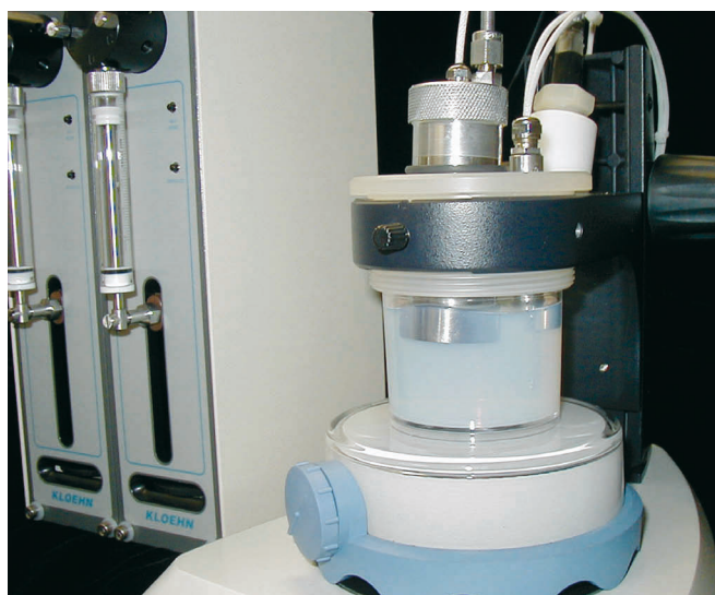
Figure 2 a-b The DT-1200 as the unique analytical instrument for characterization of concentrated dispersions and the zeta potential probe DT-300 as high quality zeta potential instrument
