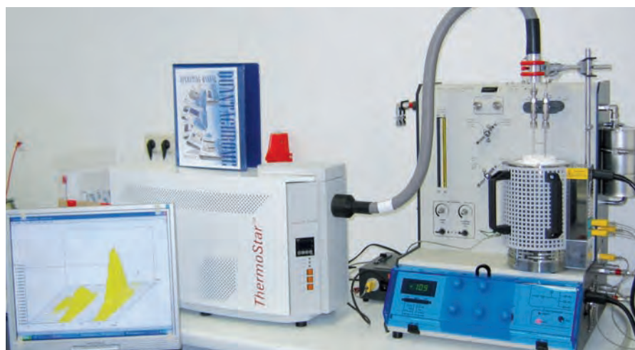
Figure CHEMBET PULSAR TPR/TPD for fully automated catalyst characterization in combination with mass spectrometer for additional determination of the reaction products of temperature programmed reactions
