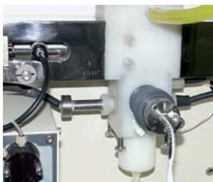
Figure 2A and B, Acoustic and electroacoustic parts of the DT-1200: Acoustic transducer (left), acoustic sensor (right), zeta potential probe (in front), smaller sensors are for temperature and conductivity measurement and for titration. The zeta potential probe can be used for external experiments, like special titrations or online-monitoring.
