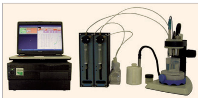
Figure 3 DT-310 instrument from DISPERSION TECHNOLOGY for zeta potential studies of complex suspensions in original concentrations
