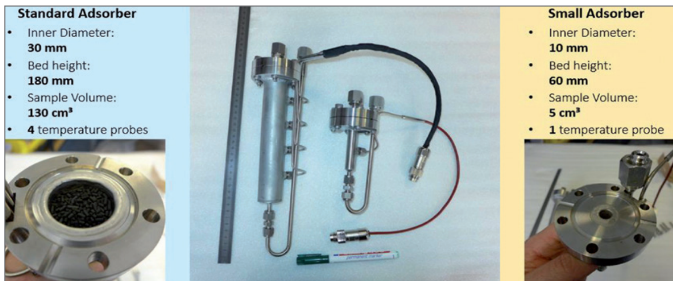
Figure 2 The mixSorb L instrument offers flexible adsorber volumes, standard adsorber with 130 ml (left) and small adsorber with 5 ml volume (right), the mixSorb S is optimized for MOFs and similar materials, its adsorber cell is for samples below 1 ml bulk volume
