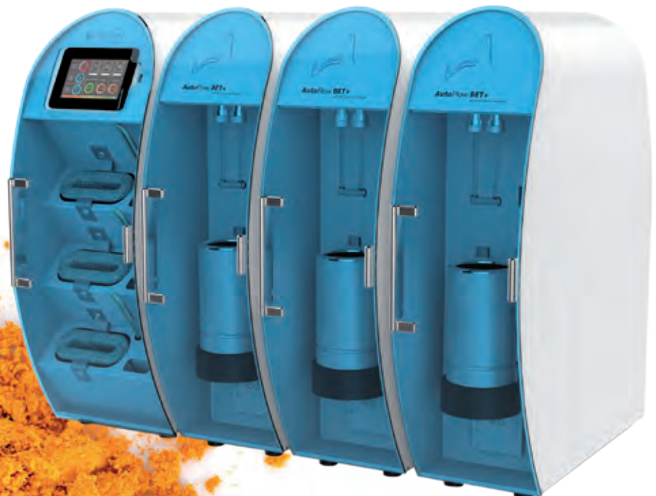
Abbildung 3 AUTOFLOW BET+ with control unit and three sample preparation stations (left) and maximum three measuring stations (right)
