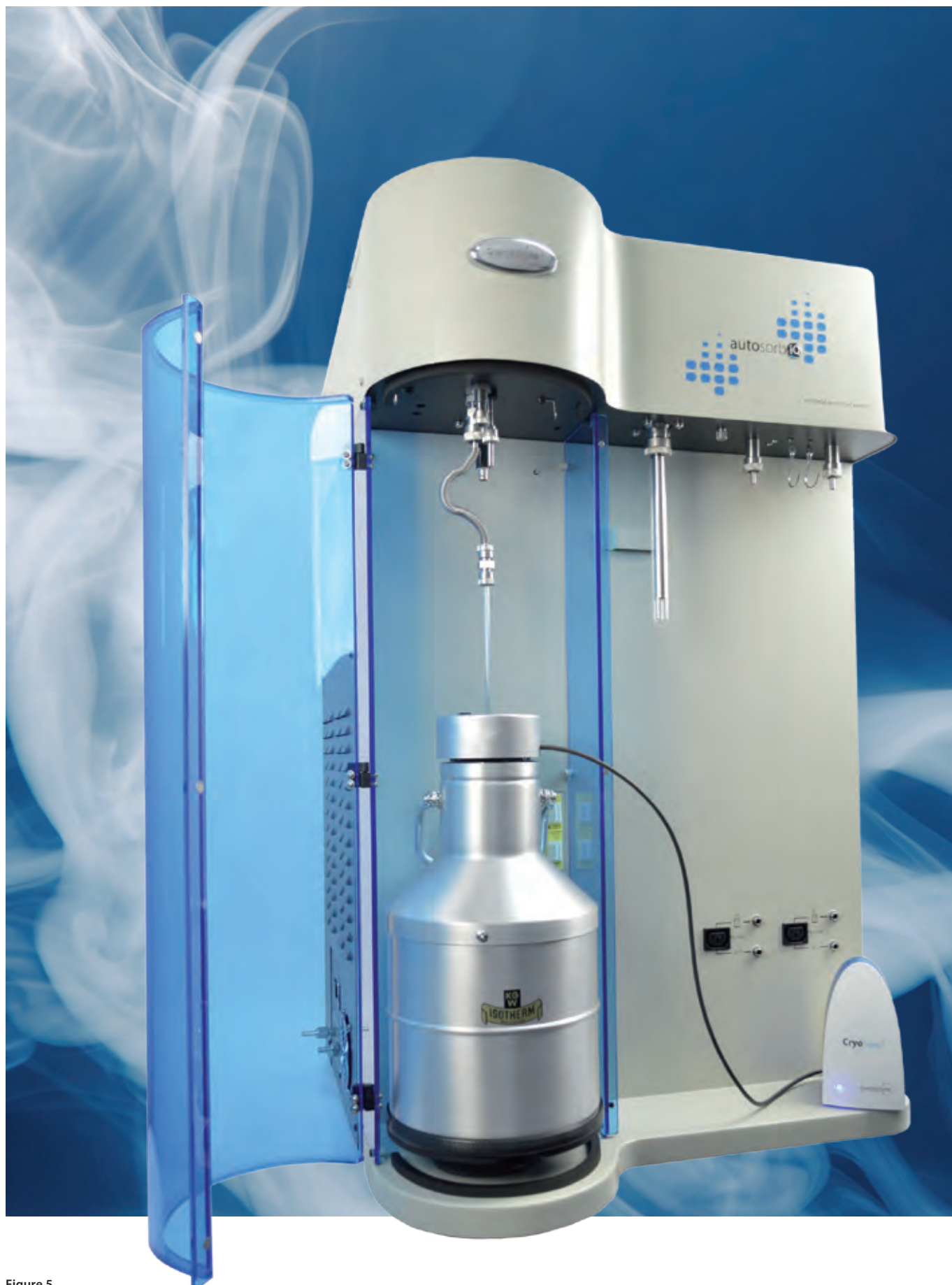
Figure 5 AUTOSORB-iQ-MP with integrated CryoSinc: CryoSinc is located in the Dewar vessel, the small controller is visible to the right, and the temperature is controlled using a PC software, CryoSinc basically does not require additional laboratory space, operates completely silently and has a power consumption of max. 30 watt
